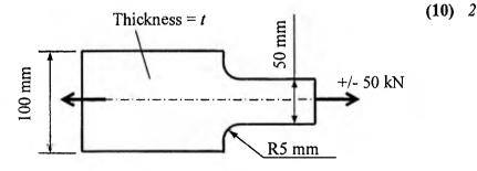
reversed axial force of 50 kN. For fatigue calculations, consider factor of safety as 2.0, notch sensitivity factor q = 0.8, size factor  $K_b = 0.85$  and reliability factor  $K_c = 0.9$ . Determine the plate thickness t for infinite life.
